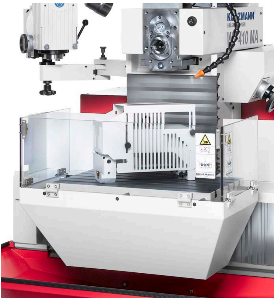
← WF 410 MA with Plexiglas splash protection, arbor holder, horizontal spindle
